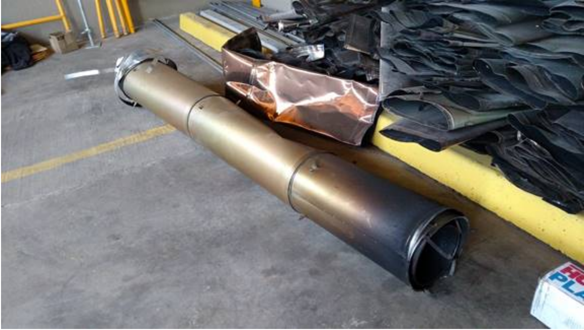
Figure 5 - evidence that a flue pipe was not well connected to the fireplace (very dangerous)!
